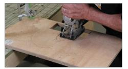
• Following the outline of the drawn shape, cut the opening into the piece of plywood.
